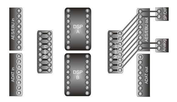
Different versions of the H8000FW support a wide range of possible outputs, as described in the chart below. Be aware that, as described above, the external outputs must be fed from the *MAIN Outputs* block.
