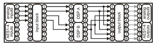
Analog inputs 1&2 are sent to DSP A, the output of which is sent to the first two analog and digital outputs. Analog inputs 3&4 are sent to DSP B, the output of which is sent to analog and digital outputs 3&4.
