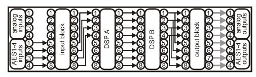
DSP B feed both the analog outputs and the digital outputs.
