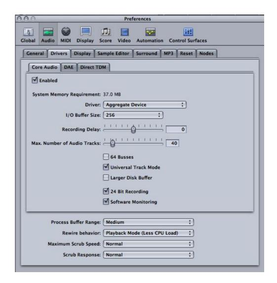
• From the **Driver** drop-down list, select **Aggregate Device** (as shown above).
