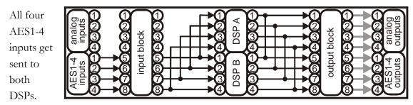
The first four outputs of each DSP are summed before being sent to the analog and AES1-4 outputs.
