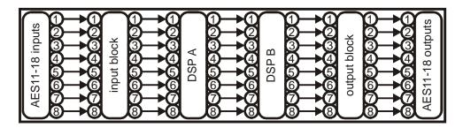
DSP B. The outputs from DSP B go to the output block, feeding the outputs.
