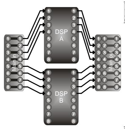
This example shows *DSP A* and *DSP B* as two separate four channel units, with *DSP A* using the first four channels and *DSP B* using the second four.
