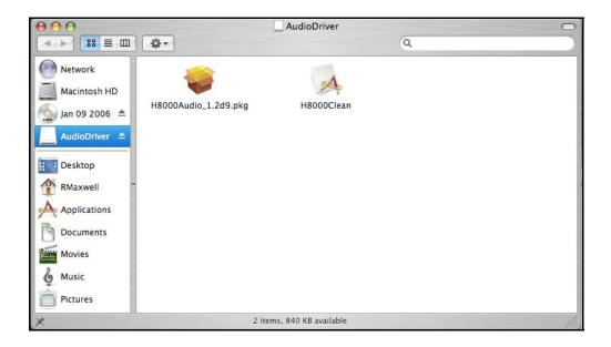
If your computer has a previous installation of H8000FW drivers, they must be removed prior to installing the new drivers. Click **H8000FWClean** to perform this action.
