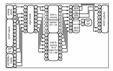
inputs. Further, assume you've loaded Backward Garden on DSP A and you want to use it to effect a monophonic, pre-amplified guitar that's being played into stereo cabinets. You also want to record the Backward Garden effect to ADAT channels 7 and 8. Our routing configuration looks like the diagram above. Note that H8000FW extra inputs and outputs are not shown, in the interest of making it remotely readable.
