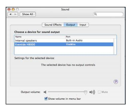
After selecting the Output tab, **Eventide H8000FW** displays as an output device, along with its port type, **Firewire**. Highlight it to select it as your output device and to override the default output device on your computer.
