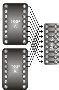
Here we have DSP A 5-8 feeding *MAIN Output* channels 5-8 (Digital)
