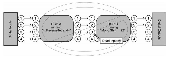
Those DSP inputs or outputs that are *not* used by the program are "dead" - no signals are passed by them. Knowing which inputs and outputs a program uses can affect which
