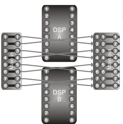
This example shows *DSP A* and *DSP B* entirely bypassed, with *Main in* feeding *Main out*, with alternate channels exchanged.
