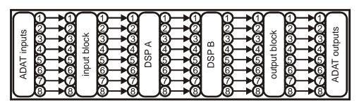
DSP B. The outputs from DSP B go to the output block, feeding the outputs.
