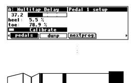
toggle between the two). The horizontal bar graph at the top of the menu page represents the current foot pedal position relative to the calibration.
