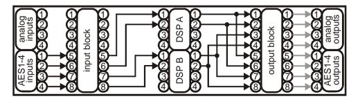
AES/EBU inputs 1&2 are sent to DSP A, the output of which is sent to the first two analog and digital outputs. AES/EBU inputs 3&4 are sent to DSP B, the output of which is sent to analog and digital outputs 3&4.
