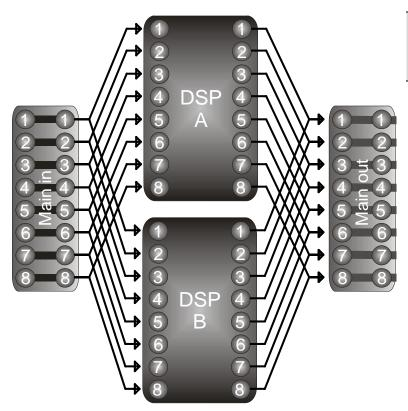
This example shows *DSP A* and *DSP B* running in parallel, both being fed from *Main in* and their outputs being mixed at *Main out*.
