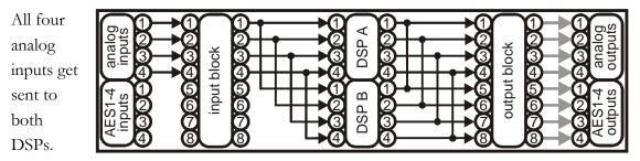
The first four outputs of each DSP are summed before being sent to the analog and AES1-4 outputs.
