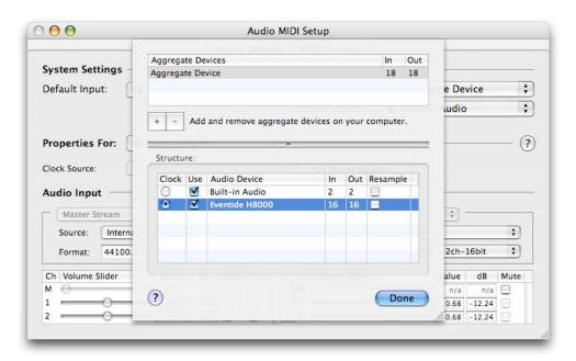
At the top of the screen, the aggregate device, comprised of the two audio devices we selected, displays, with its total number of input and output channels. At the bottom of the screen each individual audio device is listed, with its input and output channels capacity.
