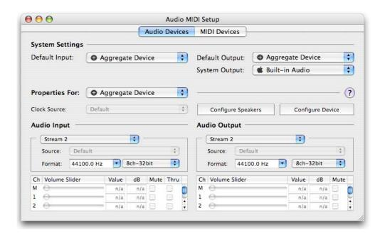
You may view the setup of the Aggregate Device by clicking the **Configure Device** button.
