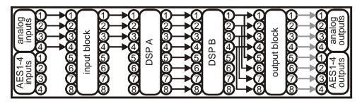
output from DSP A goes into DSP B, the output from DSP B goes into both the analog outputs and AES 1-4.
