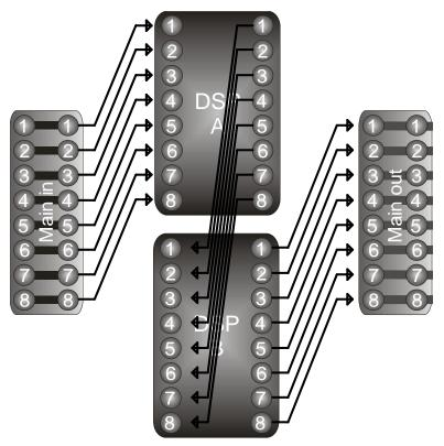
This example shows *DSP A* and *DSP B* running in series with *Main in* feeding *DSP A* which feeds *DSP B*, whose outputs feed *Main out*.
