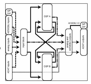
Next, "sources" are assigned to the four analog and four AES/EBU outputs (dot-dash arrows in the diagram). Again, the available sources are:
