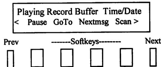
2 - You can use the hard **“Fast Forward”** and **“Rewind”** keys to move through the recorded audio at two different speeds. (Each time you depress the hard key the next fastest speed will be selected). You may also use the soft **“Next Message”**, or **“Play/Pause”** keys. The top line of the menu displays now reads **“Playing Record Buffer”** along with the Hour, Minute, Second, Day, Month, and Year.
