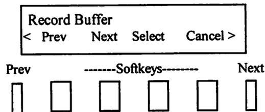
3 - Use the "Next/Previous" soft keys until you see "Record Buffer" in the top left-hand menu display. Press the "Select" soft key. The main record buffer on the hard disk is now selected for search and playback.
