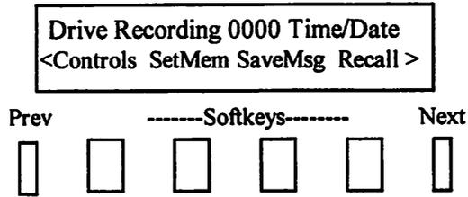
1 - While the VR 240 is in the **“Record”** mode a **“SaveMsg”** soft key is displayed. Depressing that soft key will activate the menu prompt **“What Channel?”**
