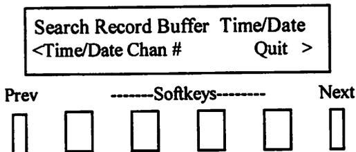
1 - If you press the **“Go To”** soft key the top line of the menu display reads **“Search Record Buffer”**. The **“Time/Date”** and **“Channel #”** soft keys are also displayed.
