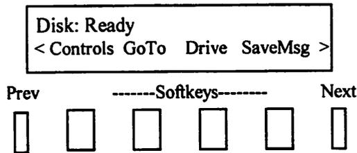
1 - Use the "Next/Previous" screen keys to locate the "Drive" soft key on the main menu display. Depress the "Drive" soft key until you see "Disk" in the upper left-hand corner of the display.
