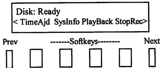
2 - Use the "Next/Previous" screen keys to find "Playback" on the menu display. Press the "Playback" soft key.
