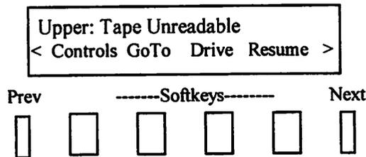
1 - Load a new tape into the drive. When loading is complete the display will read "Tape Unreadable". Press the "Next" hard key until you see "PrepTape" in the display.
