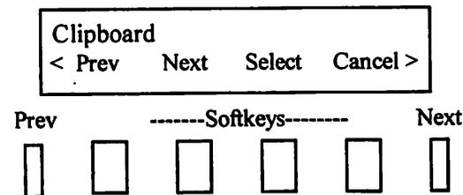
1 - Use "Next/Previous" screen keys to find "Playback" soft key. Press the "Playback" soft key and use the "Next/Previous" soft keys until you see "Clipboard" in the top left-hand side of the menu display. Press the "Select" soft key. The hard disk "Clipboard Buffer" is now selected for playback. All of the playback functions described in "Direct Playback" are now available.
