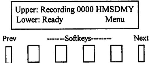
1 - To enable live monitoring press the “Menu” soft key.
