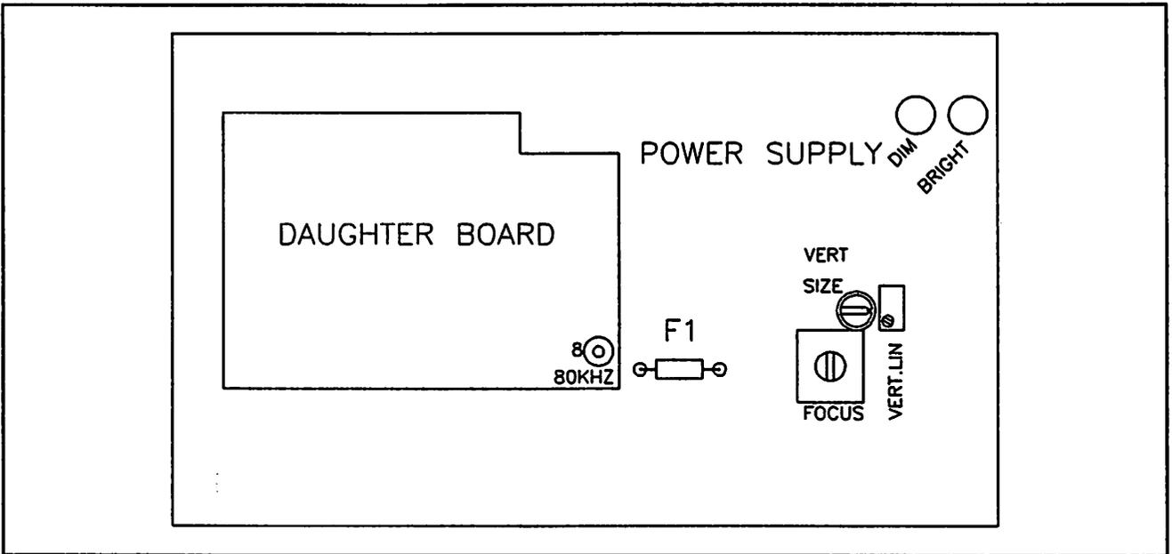
**Figure 16 - Location of Display Adjustments on Main Power Supply Board.**
