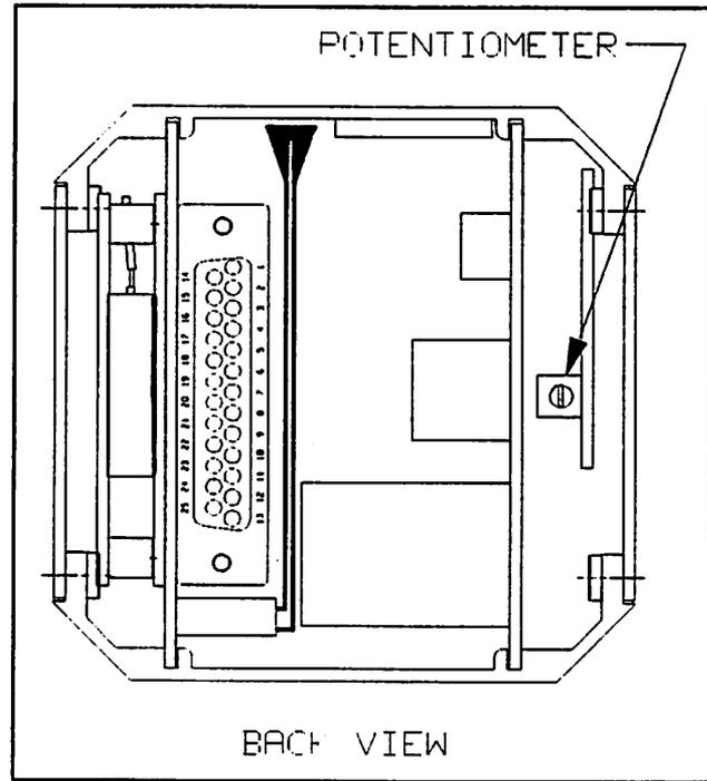
**Figure 10.** Location of Potentiometer on 3000 & 5000.
