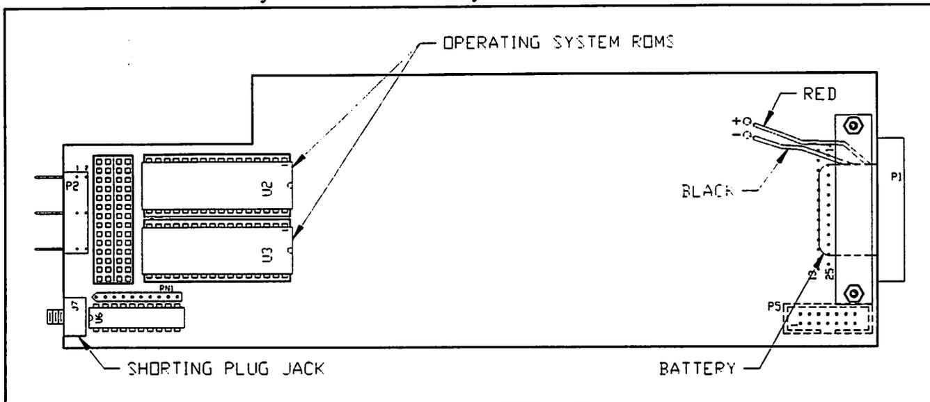
**Figure 7:** Location of Shorting Plug Jack on 5000 and 7000 CPU Board.
