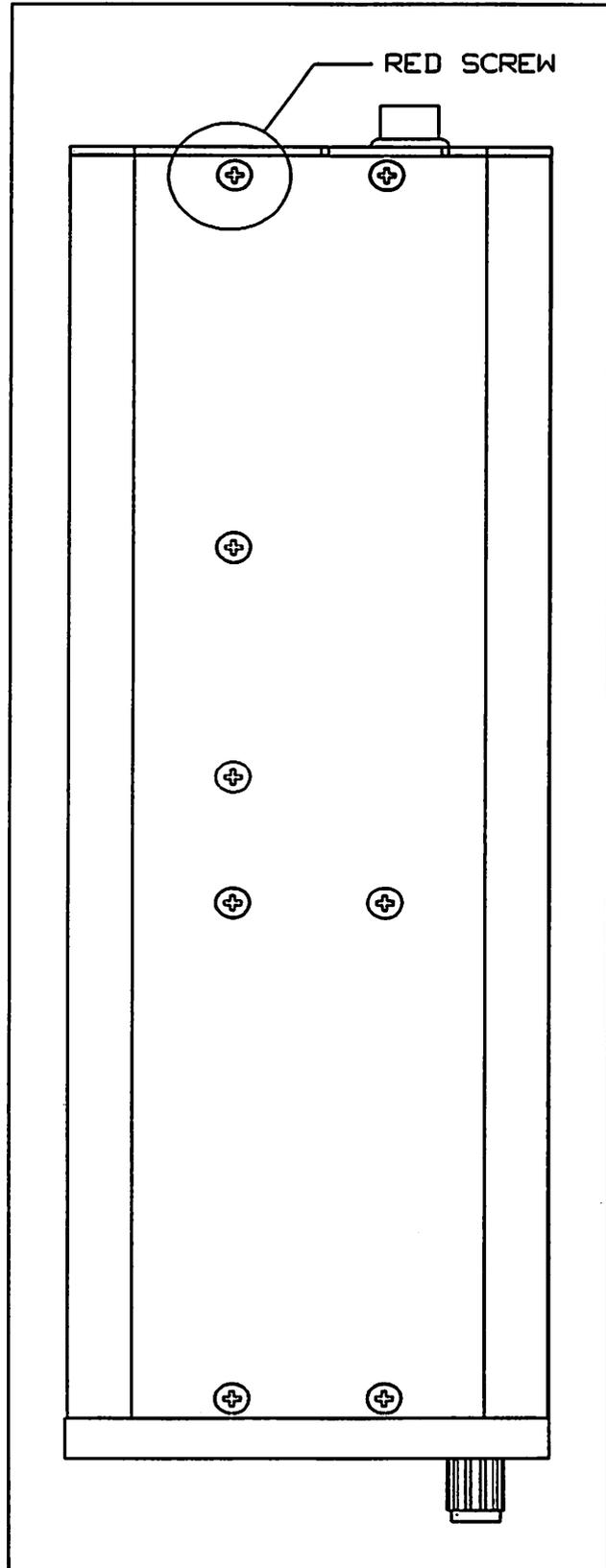
**Figure 9. Proper Placement of Red-Marked Screw on Models 3000 and 5000.**
