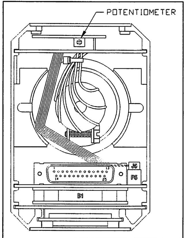
Figure 11. Location of Potentiometer on 7000.
