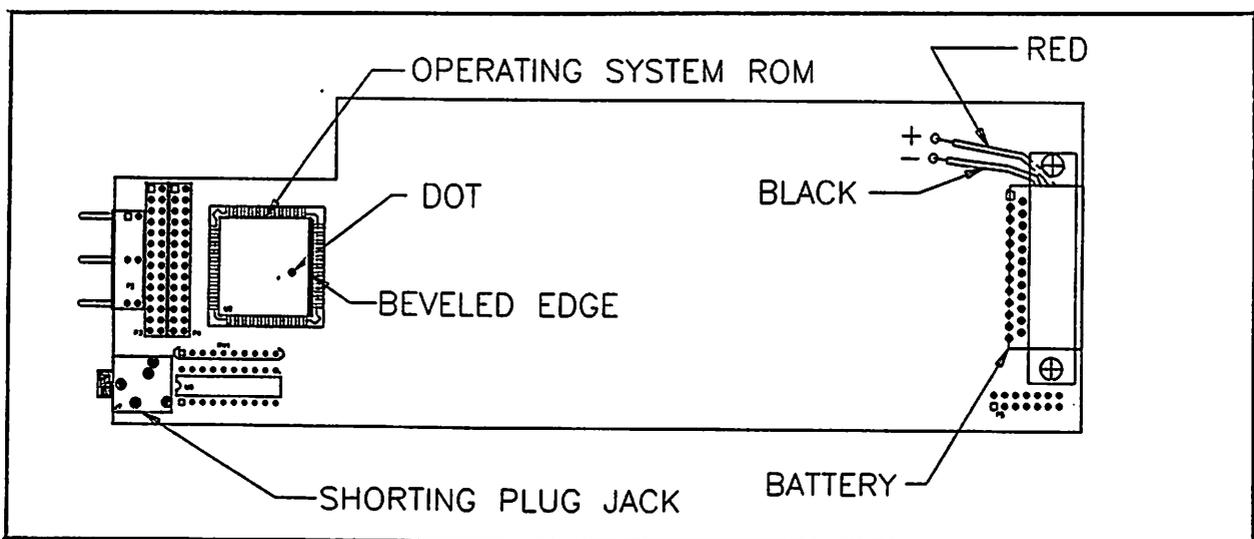
Figure 5a. ROM location on single-ROM CPU boards.
