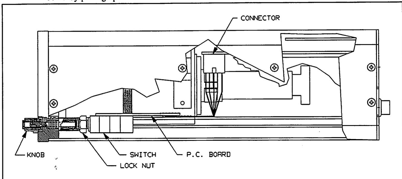
**Figure 13. ON/OFF Switch Assembly in 3000 and 5000.**
