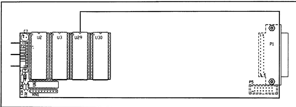
**Figure 2.** Location of ROM Chips on 3000 CPU Board.
