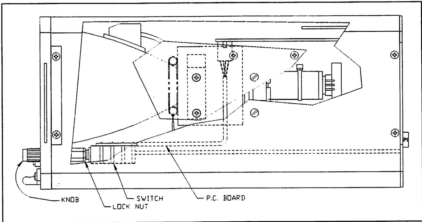
**Figure 14. ON/OFF Switch Assembly in 7000.**
