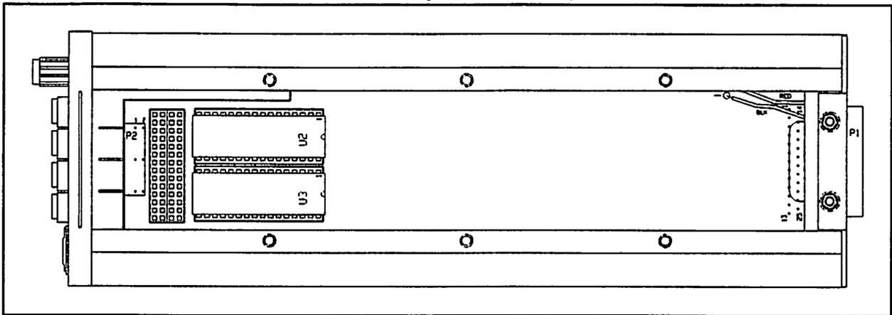
**Figure 3.** Location of ROM Chips on 5000 CPU Board.
