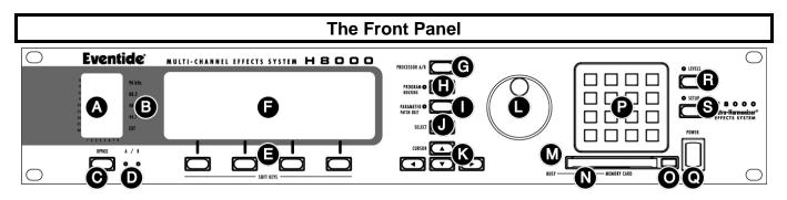
**A)** Level Meters These measure the eight signals selected for input, DSP A's eight inputs, DSP B's eight inputs, DSP A's eight outputs, DSP B's eight outputs, or the eight AES/EBU outputs (from which all of the other outputs are derived).  $\rightarrow$  See <u>The Level Meters</u> on page 47.
