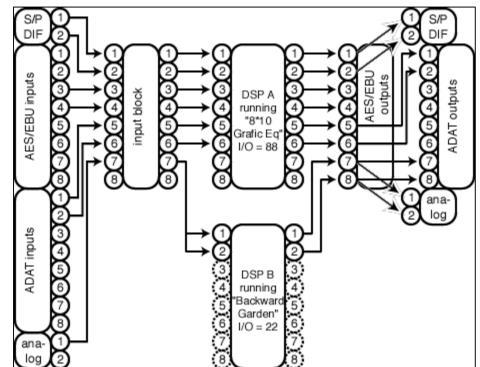
record the Backward Garden effect to ADAT channels 7 and 8. Our routing configuration looks like the diagram above.
