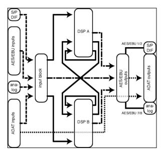
Next, "sources" are assigned to the main AES/EBU outputs (dot-dash arrows in the diagram). Again, the available sources are:
