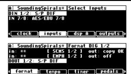
present at both the AES/EBU 1/2 output and the S/P DIF 1/2 output, but they can only be one *format*. S/P DIF selects a "consumer" format while AES/EBU selects a "professional" format. Use the AES/EBU format unless you have a compelling reason to do otherwise.
